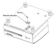
3 Slide the mounting plate lock outward and lift the mounting plate from the printer.
