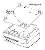
4 Using a 3 mm hex driver, remove the four screws and the mounting post bracket. Once removed, proceed to the "Install the Printer Mount" on page 3.
